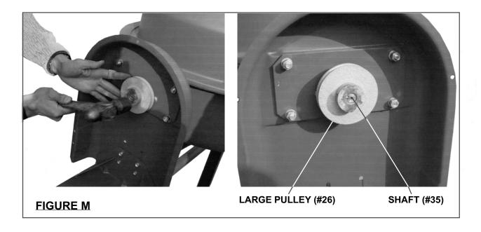
17. Loop the V-Belt (part #22) around the Large Pulley (part #26). Set the gasoline Engine (part #14) on the Engine Mount Plate (part #12) with its Small Pulley (part #16) facing the Inner Cover (part # 23). Then, loop the V-Belt around the Small Pulley. (See Figure N.)
